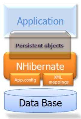
This diagram shows NHibernate using the database and configuration data to provide persistence services (and persistent objects) to the application.
